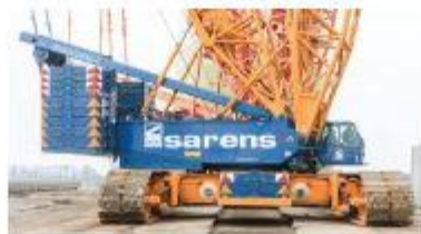
This behemoth is a Demag CC2800 with a maximum capacity of 660 tons.
