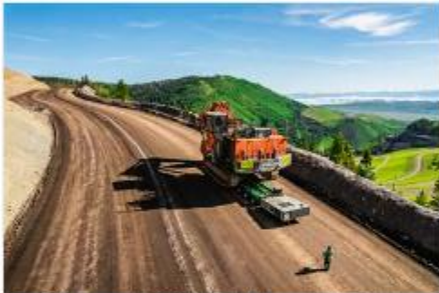
Omega Morgan moved a 500,000-pound, fully assembled Hitachi mine shovel using 10 lines of TII K25 SPMT. PHOTO: Omega Morgan
