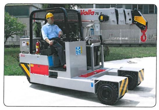
**DRIVE:** DC 8 kW - 48 V fanned, reversible electric motor with MOSFET electronic control HF and energy saving, self diagnostic, speed and temperature checks (no. 2 thermostasts), brush wear warning.
