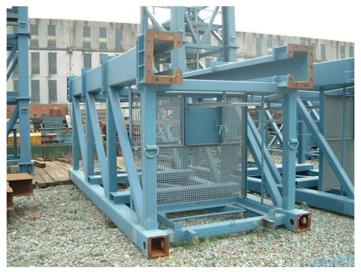
A mast of 6050 mm is built up out of 4 vertical members which are braced by means of diagonals and K bracings. The back panel vertical members are RHS 250 x 12,5 sections and the front panel vertical are the piston guides. All diagonals and braces are RHS profiles.
