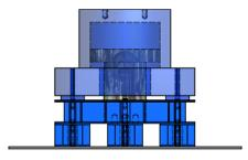
Phase 7: The jacking cylinder is re-energised; thus retracting its cylinder. The load is transferred on the 2 newly
