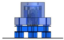
Phase 8-9-...: The jacking cylinder is energised; thus extending its ram, pushing up the jack & transferring the
