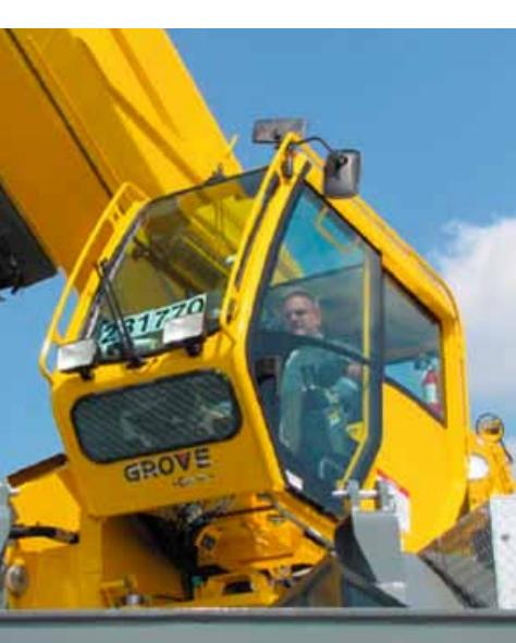
• **Full vision cab:** New full-vision cab, all-steel fabricated with acoustical lining and tinted safety glass throughout. The cab tilts up to 20° providing the operator additional comfort when working at long boom and extension lengths.
