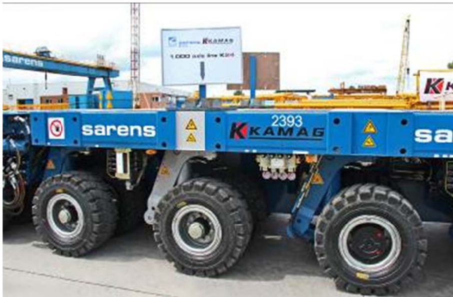
Axle line number 1.000 KAMAG K24 modular transporter at Sarens, Belgium
