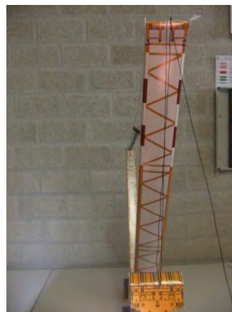
To thread the hook, 2 cables are needed. The length of one cable is approx. 20 times the desired distance between the boom head and the hook.
