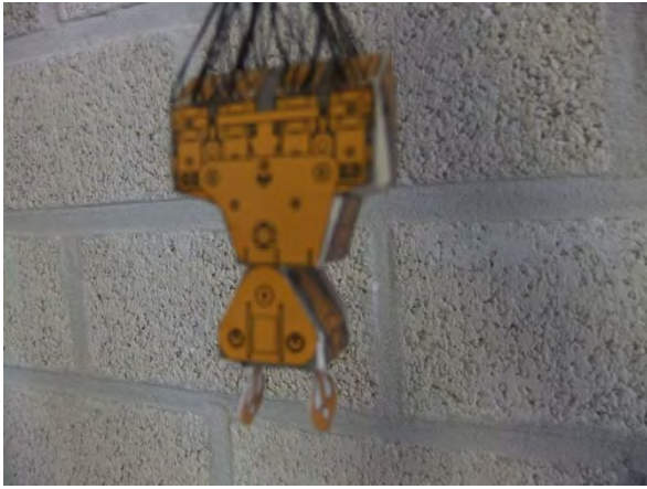
The hook block completed
