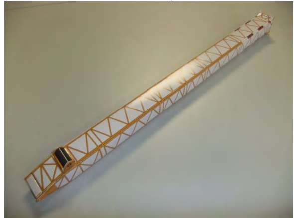
The main boom completed with hinge, main boom head, winch and reinforcement box
