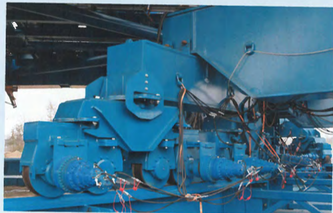
▲ A total of sixty-four type A2FM hydraulic motors drive the slewing mechanism for this giant.
