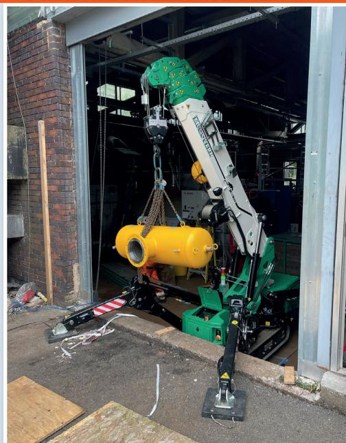
The angles and orientations of the crane's outriggers can be adjusted to suit the site
