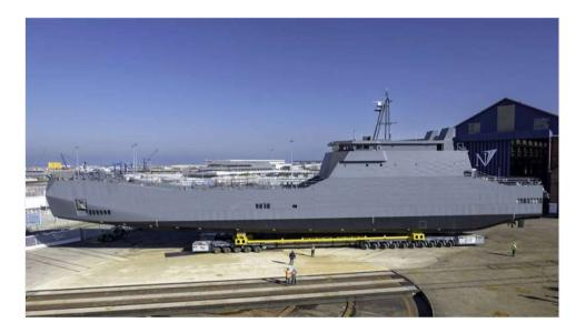
Sarens selected the equipment for this operation for its ability to masterfully move the vessel from the CMN factory to the Syncrolift lifting system at the ferry terminal, and also to successfully carry heavy loads over short distances. The crane and SPMTs were mobilised to the site via nine trucks and required one full day for rigging.
