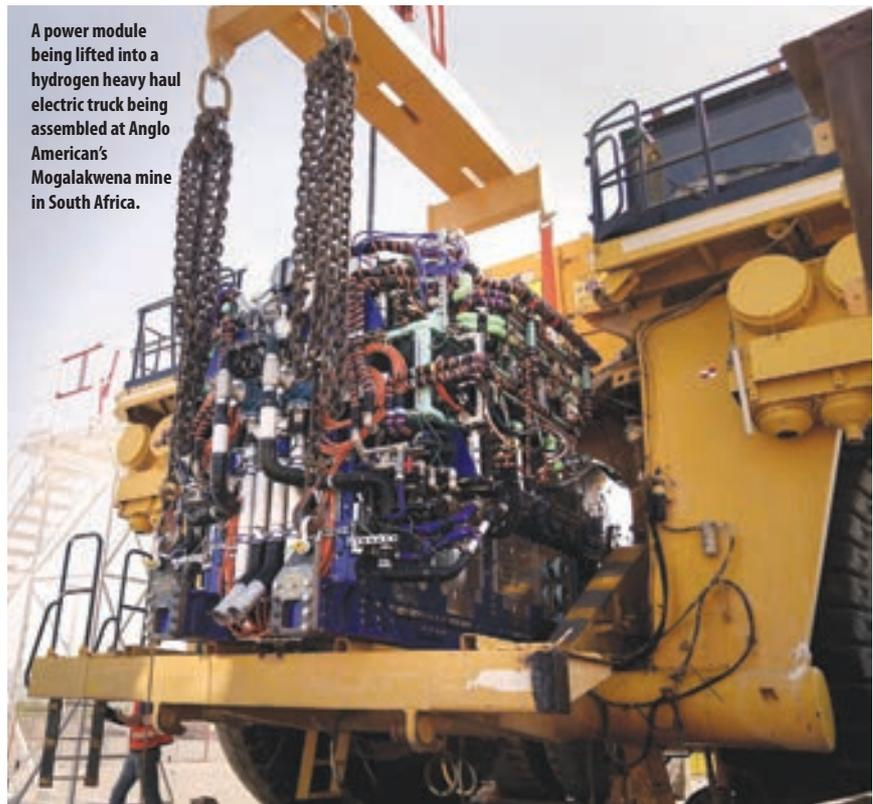
A power module being lifted into a hydrogen heavy haul electric truck being assembled at Anglo American's Mogalakwena mine in South Africa.
