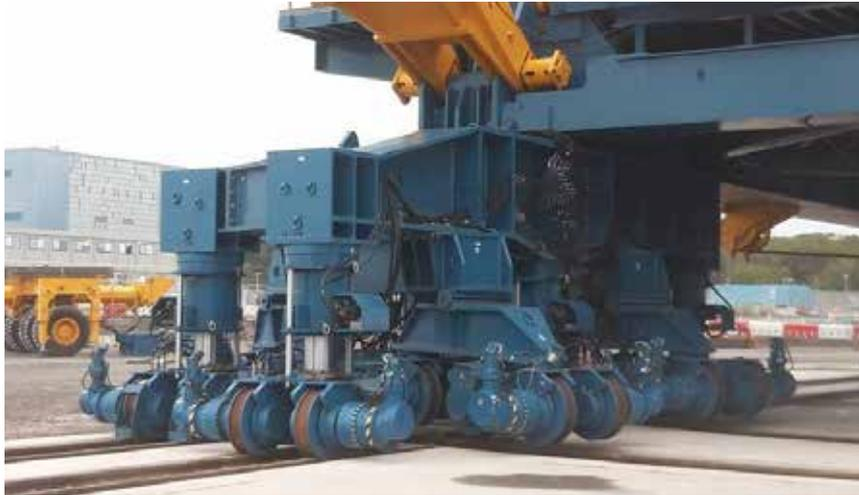
For 360° slewing and lifting operation, the SGC-250 is positioned on the ring. With hydraulic cylinders the SGC-250 can switch from ring to straight rails.
