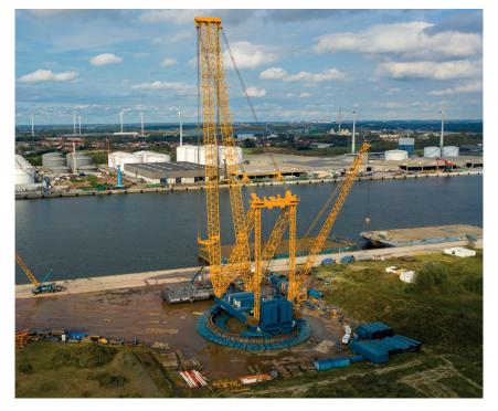
produce its own energy, recovering and reusing the electricity it generates each time it lowers a load. When connected to the national grid, it recovers all produced energy and feeds it back, reducing energy consumption by up to 40%," said the heavy lift specialist.
