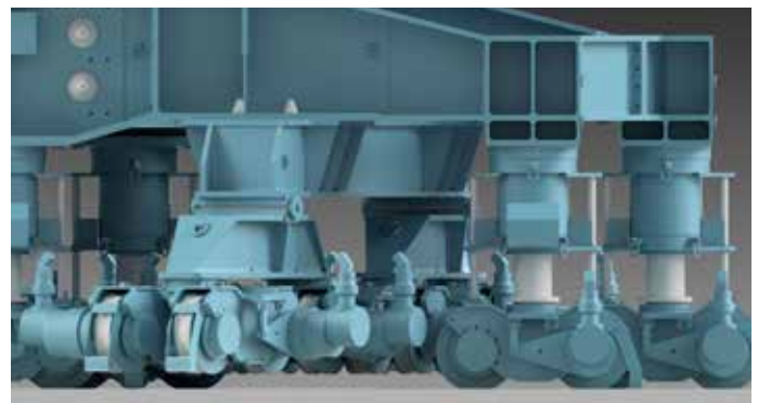
SGC-250 supported on 96 wheels cylinder fully extended
