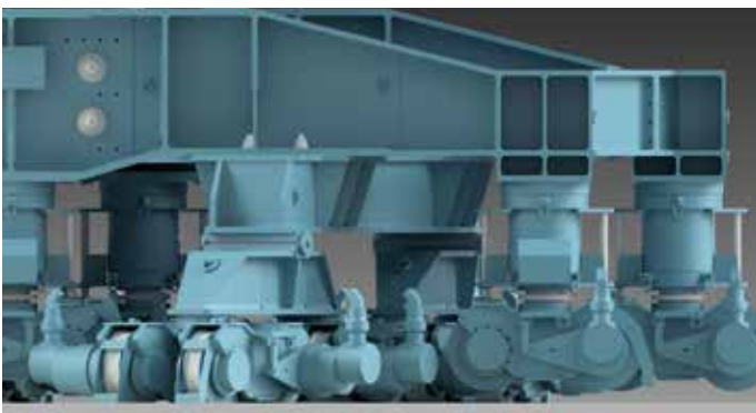
SGC-250 supported on 128 wheels cylinder retracted
