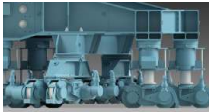
SGC-250 supported on 96 wheels cylinder fully extended
