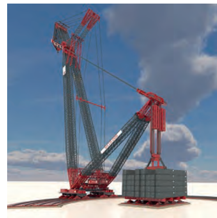
ALE's 10,000 tonne capacity AL.SK10,000 super heavy lifter
