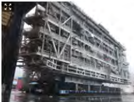
Sarens using Kamag SPMT on Johan Sverdrup oil field module
