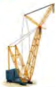
Sarens SGC 250 super heavy lift ring crane
