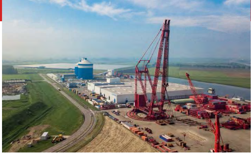
Mammoet has increased the capability of its 200,000 tonne-metre class PTC 200 DS ring crane
