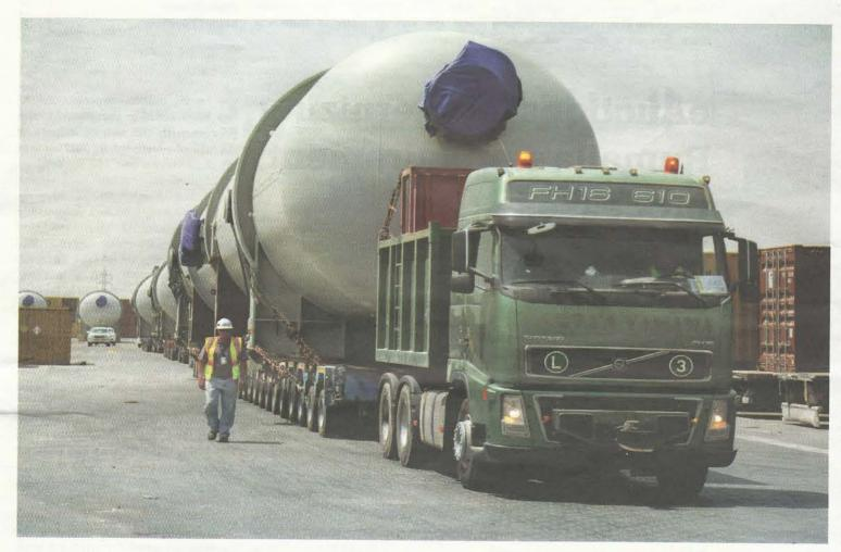
A new electrostatic desalter vessel has arrived at Rumaila, in an operation which has been described as one of the largest shipments ever to be moved on Iraqi roads.
