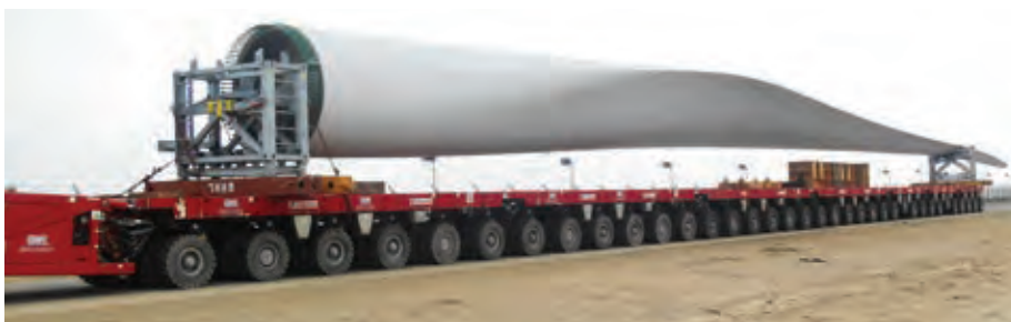
36 axle lines of Scheurle SPMT were used to move three 58 metre long rotor blades for the Gulf Haulage Heavy Lift Company (GHHL) in Saudi Arabia
