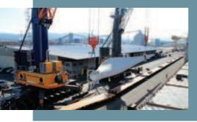
tandem, wind turbine blades were discharged directly from the vessel to rail cars. This, the port said, provided both time efficiencies and cost savings to its customer. The 160 foot (49 metre) blades, manufactured by Vestas, were discharged to flat-bed rail cars adjacent the vessel, moving along the port's on-dock rail system. Each blade required two railcars which then transported them to a wind farm in Illinois.
