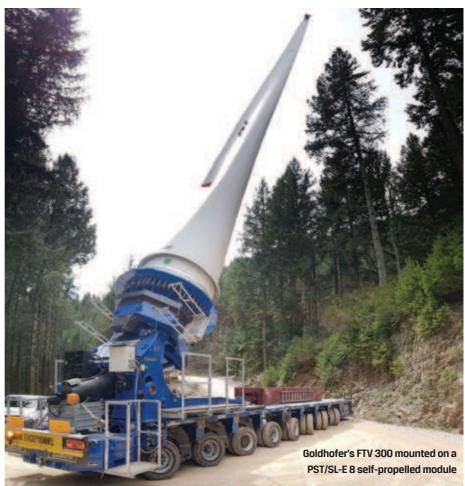
transporting long rotor blades; its RA4 tower adapter for transporting heavy tower sections (up to 180 tonnes); a range of low loaders with various axle systems for transporting nacelles; and a range of drop-deck vehicles for transporting turbine hubs designed to comply with regulations for maximum load height (which is 4.2 metres in most countries).
