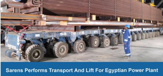
Sarens recently transported and lifted heat recovery steam generator (HRSG) modules for the New Capital power plant, a 4.800MW combined-cycle power plant
