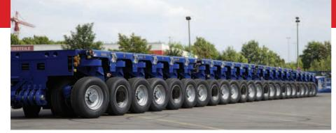
With a track width of 1,810 mm, the PST/ES-E 285 from Goldhofer has a lateral stability which is 25% higher than that of a conventional SPMT
