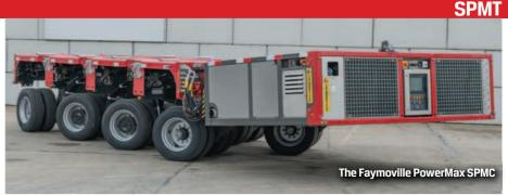
making these the world's highest capacity SPMTs. The trailers also have a much higher bending moment capacity. This enables them to have a greater spread and the ability to carry an increased loading. They have mainly been used across ALE branches in the UK and the Netherlands."
