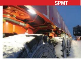
Mammoet has purchased last generation Scheurle SPMT, but with a special Arctic specification. They also have LED lighting to illuminate the area around the vehicles which is an advantage when working in areas where daylight hours are scarce
