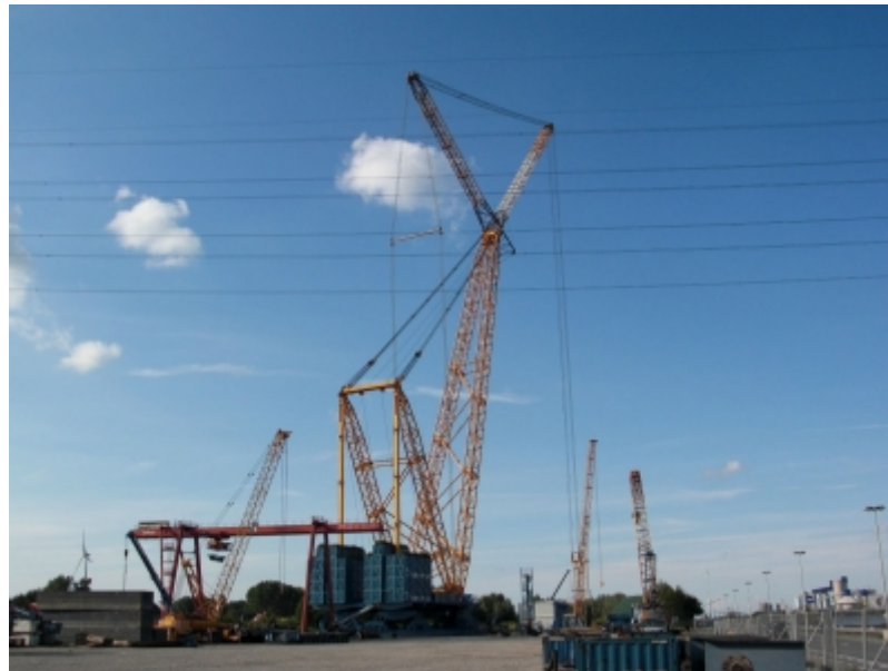
Sarens' 3,200-tonne capacity SGC 120 heavy lift crane.
