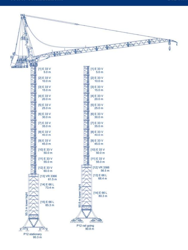
Tower combinations according to C 25 wind data.
