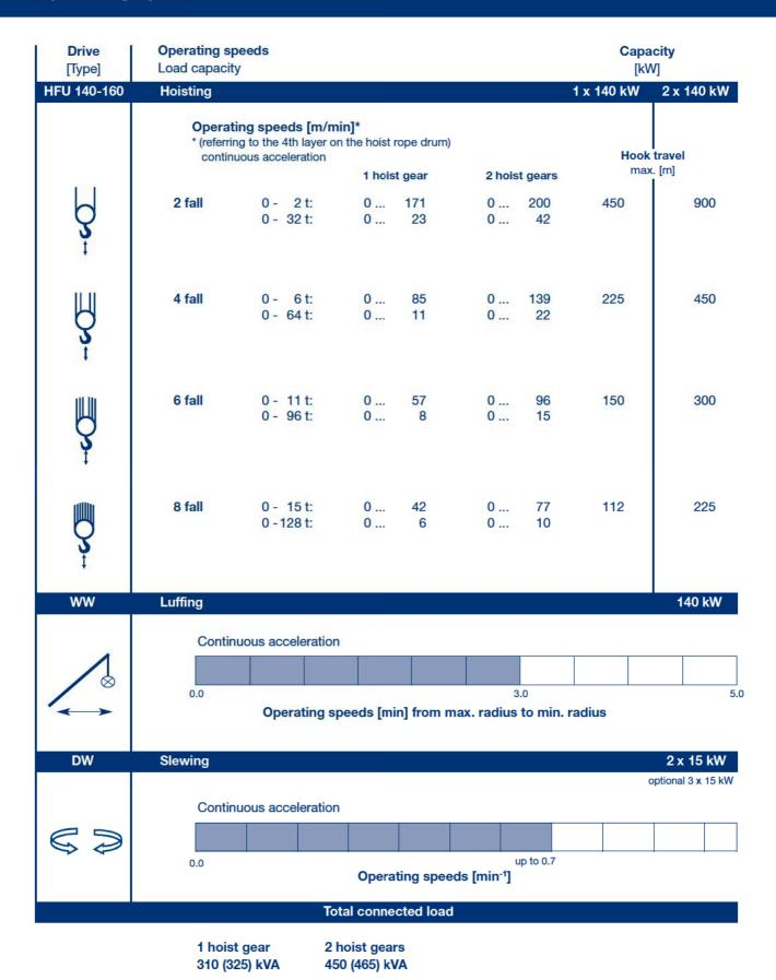
Total connected load at utilisation factor 0.7
