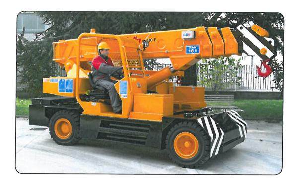
PROPULSION: 18 kW - 96 V DC fanned reversible electric motor fitted with a MOSFET speed control and microprocessor. Foot operated brakes to driving wheels and hydraulic shoe brakes on front wheels. Hand brake mechanically operated.
