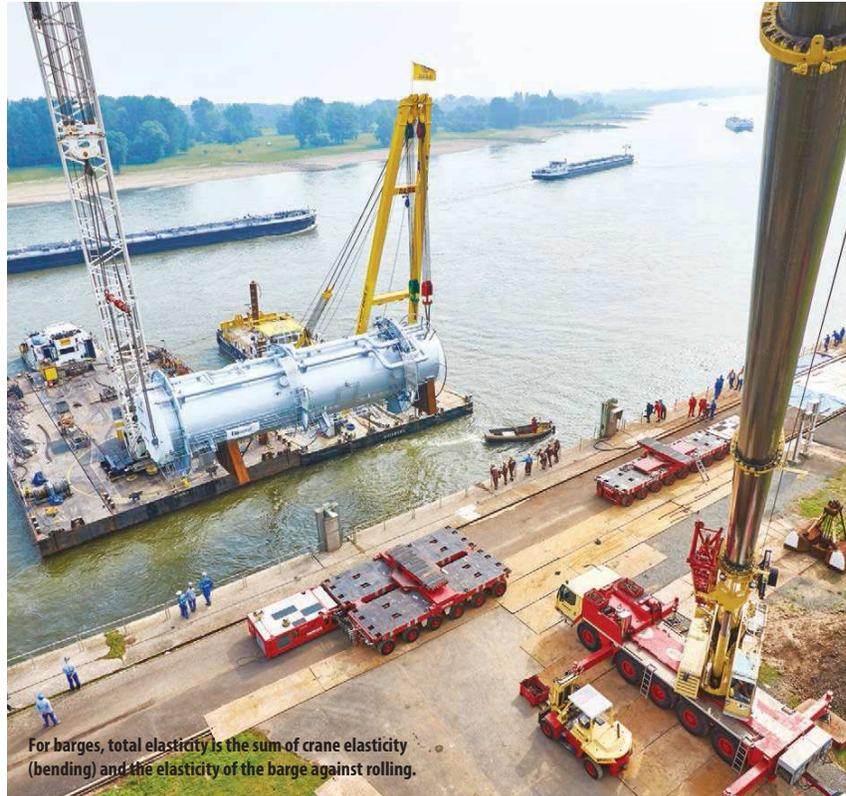
For barges, total elasticity is the sum of crane elasticity (bending) and the elasticity of the barge against rolling.
