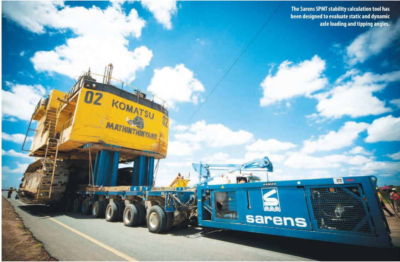
The Sarens SPMT stability calculation tool has been designed to evaluate static and dynamic axle loading and tipping angles.
