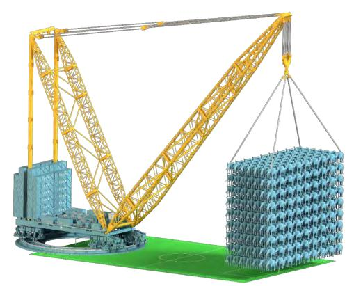
Besides power and flexibility, Sarens has put significant effort on safety and continuity. This can, for example, be seen on the highest performance level (PL E) and full redundancy system on the hoisting and slewing system which is achieved by intelligently connecting and steering all 12 engines in six power packs.
