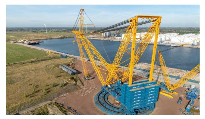
The SGC-250 is the first of the 3rd generation of ring-based cranes at Sarens. It has a maximum load moment of 250.000Tm which allows lifting an astonishing 5.000T. Even at a large radius of 100m, the crane is still capable of lifting 2.000T and, even when doing so, the ground pressure remains below 25T/m<sup>2</sup>. This extremely impressive metric is achieved through the high number of wheel bogies on the double ring beams and the spreader mats that the machine features.
