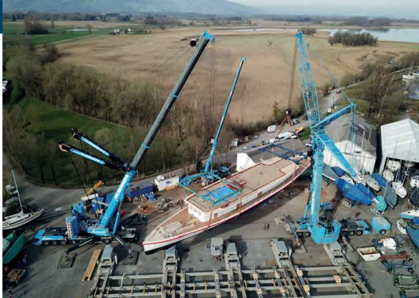
Felbermayr subsidiary Bau-Trans used a pair of mobile cranes lifting in tandem to return the historic ship MS Osterreich , built in 1928 and weighing 160 tonnes, to a slipway on an Austrian inland waterway. The 55 metre vessel was decommissioned in 2009 and almost scrapped
