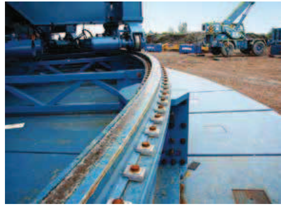
The rail tracks are bolted onto two heavy I beam supports.
