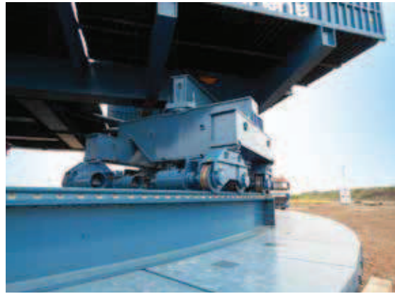
The rail tracks are bolted onto two heavy I beam supports.
