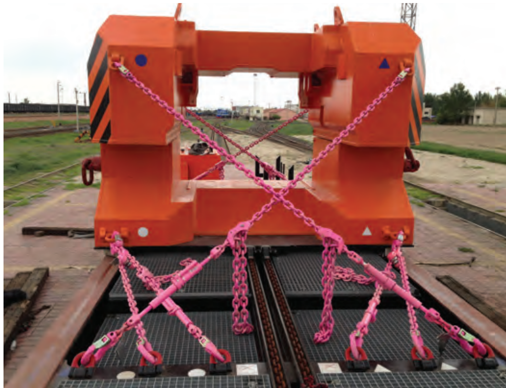
Rud utilised a 'loop-around' principle to safely secure a transport trolley and counter weight
