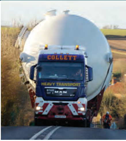
Collett transported a 28-metre-long, 140 tonne de-aerator vessel 180 km from the factory where it was built to the Port of Immingham, UK
