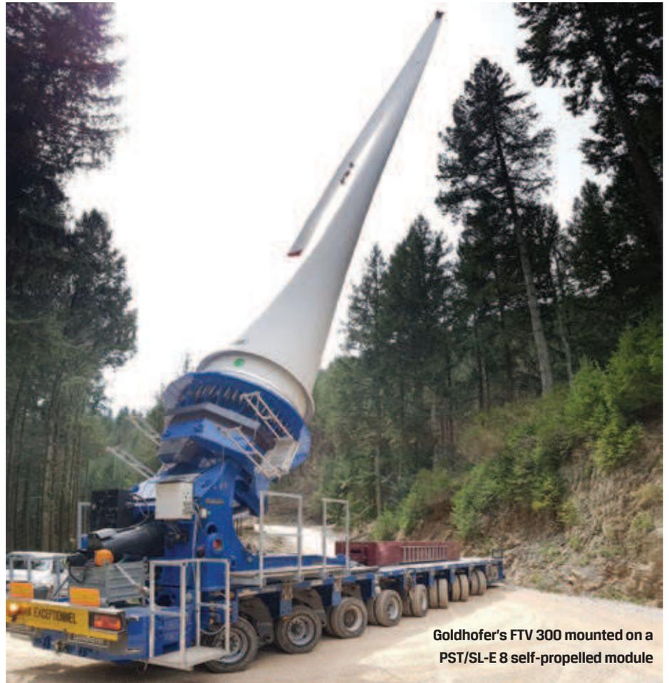
Goldhofer's FTV 300 mounted on a PST/SL-E 8 self-propelled module
